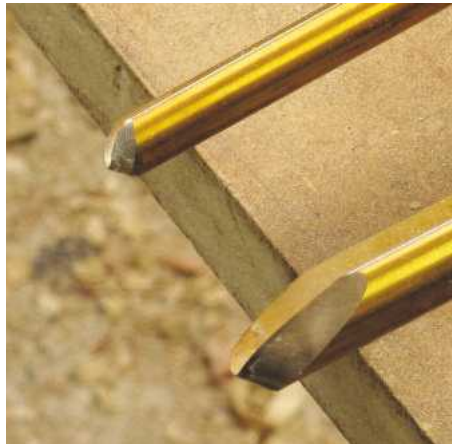
▲ Pic.2 Most of the work will be carried out with the 13mm-diameter bowl gouge with the wings of the tool ground back and the 10mm-diameter tool with a straight-across grind
